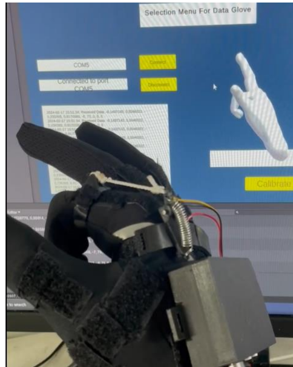
Figure 6: Data Glove using Resistive Finger Tracking - Finger Close
