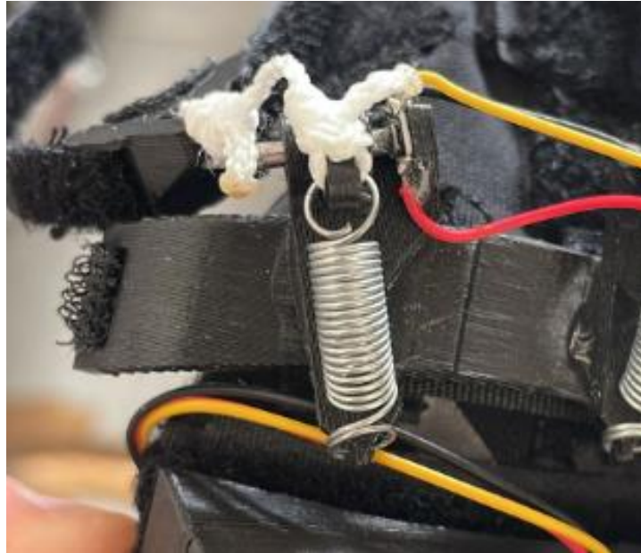
Figure 8: Resistive Finger Tracking using Potentiometers: Hardware Setup
