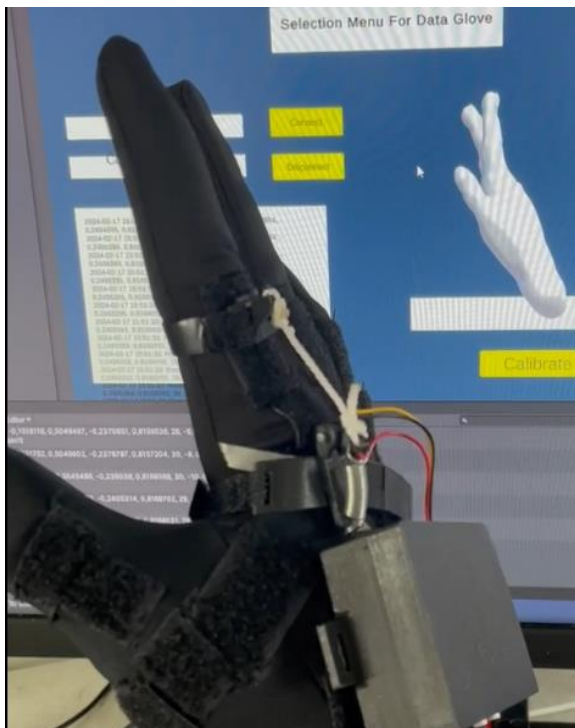
Figure 7: Data Glove using Resistive Finger Tracking - Finger Open
